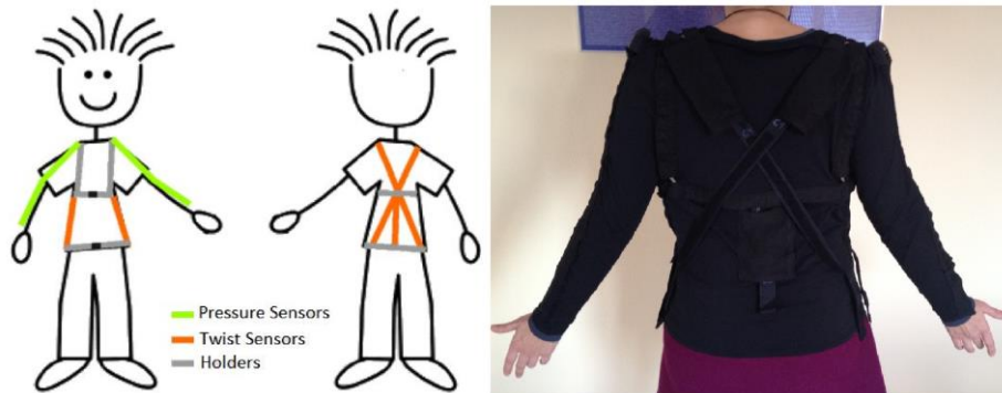
Figure 1. Representation and photo of the body sensor network which we used.
